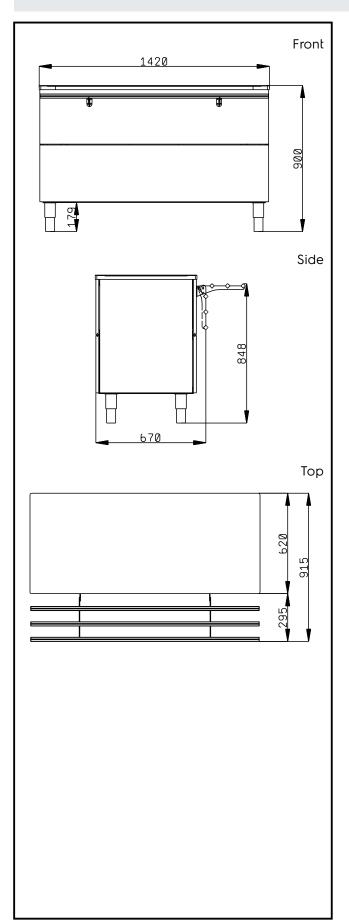
Flexy Compact Ambient Unit on cupboard (4 GN) with one stainless steel tray slider
